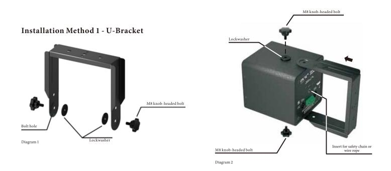
Use the large handled knob-headed bolts to mate the U-Bracket to the cabinet, placing lockwashers between the bracket and bolt. (See diagram 1 & 2 on page 4). Tighten the knob very firmly to retain the desired angle.
