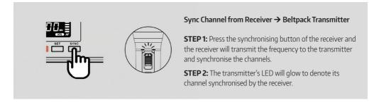
If it doesn't work check that you have the IR sensor panels aligned, that they are facing each other, devices are within 30cm of each other, and try again.
