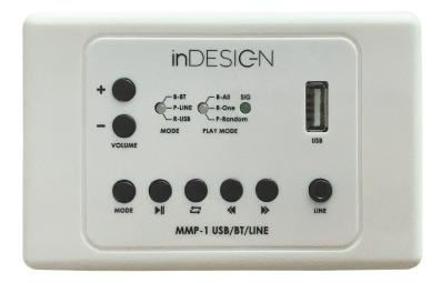
The MMP-1 is a universal remote wall panel featuring three input modes: BT, Line input and USB audio file playback. It can used as a remote input to distributed audio systems, or on its own connected directly to mixers, amplifiers or speaker systems. Users have the choice to connect the MMP-1 locally in an installed space or connect to devices remotely via inexpensive CAT6A twisted pair cabling.
