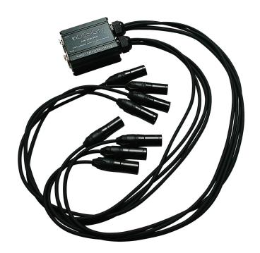
The NW-85M and NW-45F are handy tools to allow extension of audio signals over inexpensive category network cable. Send up to 4 balanced analogue or AES/EBU per CAT 6 or 7 shielded cable. A total of 8 balanced signals may be sent via 1 NW-85M and 2 x NW45F extension boxes. The extension boxes are passive, no power supply is required.
