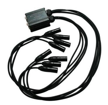
The NW-85M and NW-45F are handy tools to allow extension of audio signals over inexpensive category network cable. Send up to 4 balanced analogue or AES/EBU per CAT 6 or 7 shielded cable. A total of 8 balanced signals may be sent via 1 NW-85M and 2 x NW45F extension boxes. The extension boxes are passive, no power supply is required.
